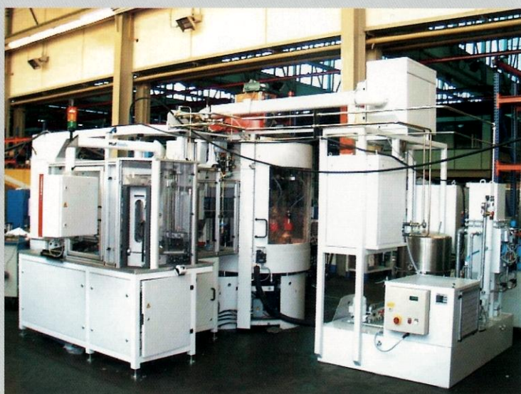
MicroStar with automation cell; bulk container into staple grid with pre- and in-process gauge as well as with SPC unit
