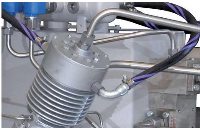
Water-cooled valve head
