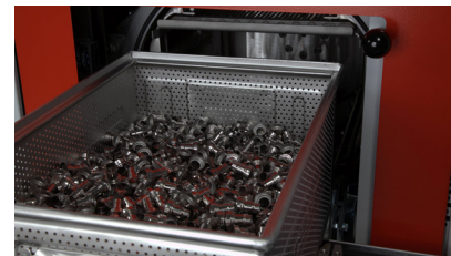
Cleaning in the goods carriers with a perforated plate
