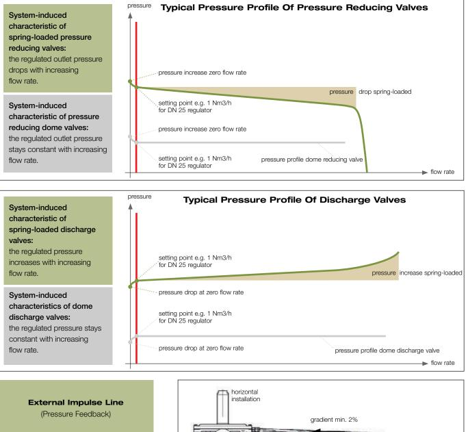
If the secondary pressure is set below 10 mbar, or are pressure losses at the pressure reducing valve outlet, e.g. due to built-in instruments, to be expected, which will exceed the set pressure at the pressure reducing valve, then external impulse line is to be considered. Also, if quickly large flow rates are demanded.
