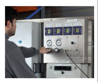
All pressure regulators are tested on our test bench for function and are set to process data. Before this function test the pressure regulators are tested for leakage to the outside. For every manufactured regulator performance data and regulator characteristics are captured.
