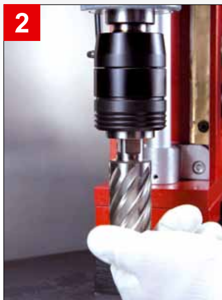
Picture 2: Insert the core drill in the EasyLock. This locks in with a loud "click." The ring spanner snaps down.
