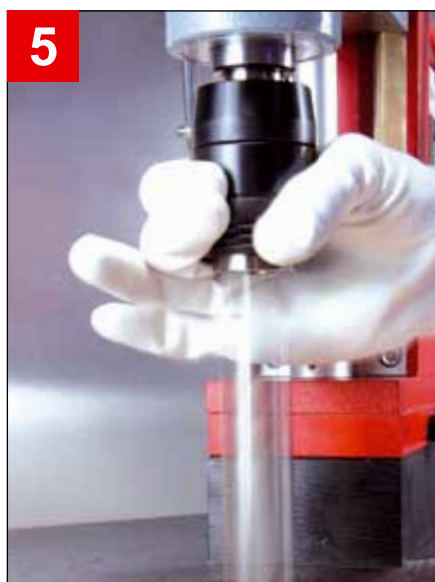
Picture 4: To release the core drill, push the ring spanner up.
