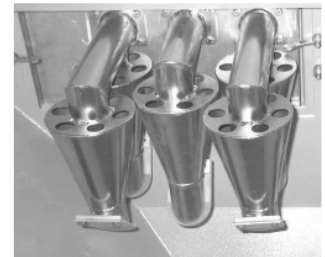
Zyklon-Anlage Cyclone installation Installation de cyclones
