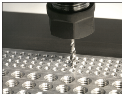
The Haas-built BT30 taper inline direct-drive spindle provides 12 000 rpm for high-speed milling, and allows rigid tapping at speeds up to 5 000 rpm.
