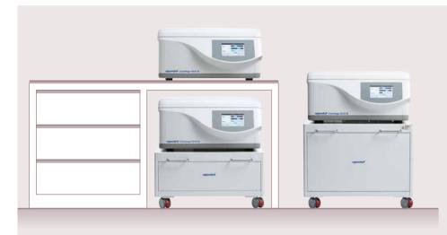
Both options come with heavy duty wheels and brakes, so you can roll them wherever you need them in your lab. To ensure your safety, they are crash-tested according to IEC 61010-2-020, offering the same safety level as stationary lab benches.
