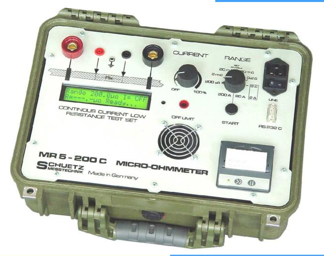
The MICRO-OHMMETER MR5-200C is used to determine electric resistances on very low - resistance objects (e.g. bus bars, any connectors) while using a very high, continous flowing measurement current. The MR5-200C is able to generate a stable maximum current • Max. resolution 0.1  $\mu\Omega$  = 100 Nanoohm up to 200 A.
