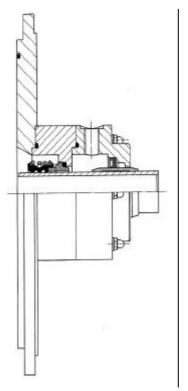
Single-acting, loaded, internal seal, independent of direction of rotation, with quenching chamber. The quenching chamber is sealed from the atmosphere by a shaft sealing ring to prevent deposits and/or reduction of the temperature in the area of the mechanical seal.
