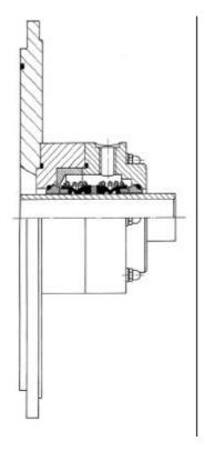
Double-acting, loaded, internal seal, independent fo direction of rotation, arranged back-to-back with sealing chamber. This arrangement is the most usual form of double-acting seals used for difficult, chemically particularly aggressive media.
