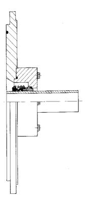
Single-acting, loaded, internal seal, independent of direction of rotation.
