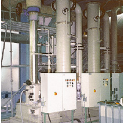
Bypass plant for recovering hydrochloric acid from flue gas
