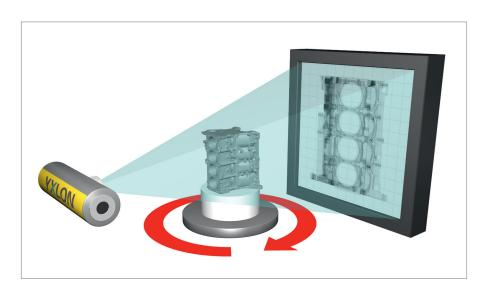
Principle of cone-beam CT: The 3D model comprises all information acquired by the detector during the rotation.
