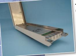
The Datapag® SolarPag system has been designed specifically to monitor the temperature of the glass substrate as it passes through the vacuum coating process. The profiling system passes through the multichamber process measuring the temperature profile from up to 4 positions on the glass; even with the plasma activated. This feature combined with the unique reflective plate thermal barrier enables the system to be used without disrupting normal production flow.
