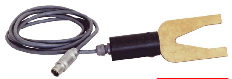
The Kelvin lug is a robust two-pole measuring contact connecting to connection and winding pins, in particular in the case of transformers, and bolted connections and busbars in power engineering applications. It is designed for practical use under rough conditions. With 2 Kelvin lugs a 4-pole connection can be realised, so that the electric resistance of the test object can be measured with a suitable measuring instrument independent of the supply line resistances.
